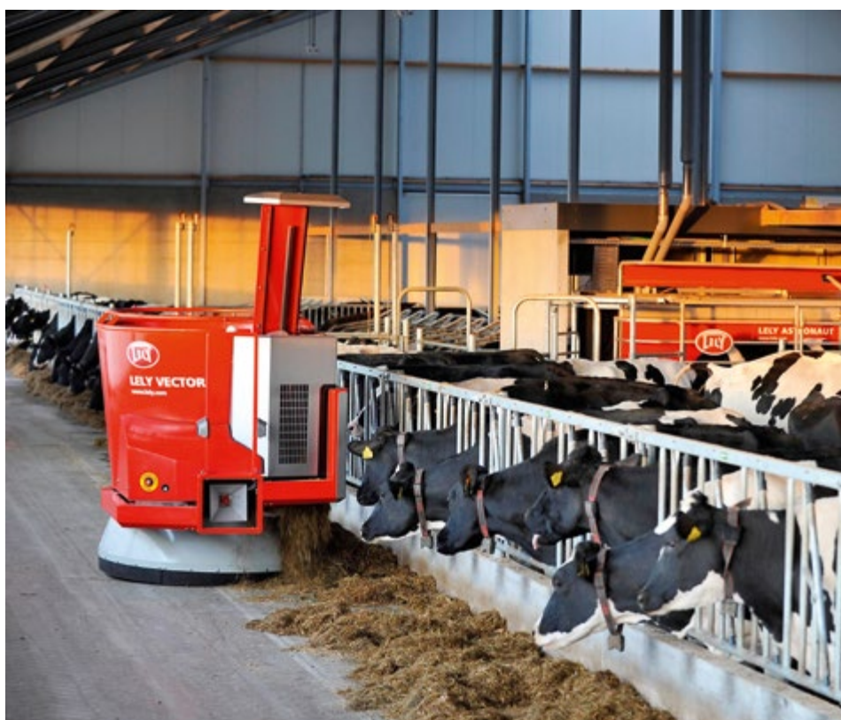
An automatic feeding system from Lely supplies cows in a barn. Small and medium-sized enterprises from the Netherlands are at the top as far as world market innovations are concerned. Many occur in the agricultural sector.
